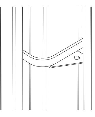
This system gives additional reinforcement to the hinge jamb and ensures that both hinges will remain perfectly aligned, even after years of heavy usage. As the door swings open, there is a massive amount of pressure and weight put on the hinge jamb. The gusset reinforces the face of the jamb that houses the hinges to the steel embedded in the concrete. The holes in the gusset serve as dowels to securely and permanently attach the gusset to the concrete.
