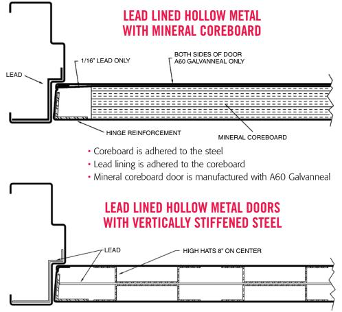
• High hats 8" on center welded to pan and cover
